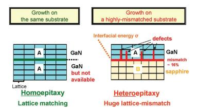
**FIGURE 6.** Schematics of homoepitaxy (ex. GaN on GaN case) and heteroepitaxy (ex. GaN on sapphire case).
