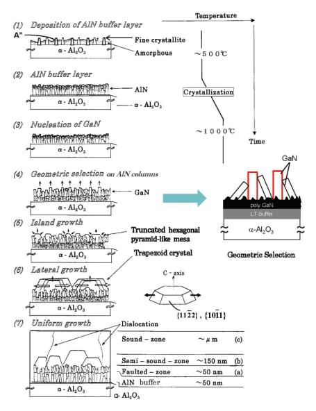
**FIGURE 13.** A growth model of GaN on sapphire with LT-buffer layer. "Geometric selection" of the GaN fine crystals was suggested.
