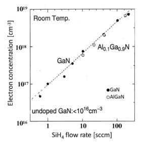
**FIGURE 15.** Electron concentrations in GaN (•) and AlGaN ( $\circ$ ) as a function of SiH<sub>4</sub> flow rate.
