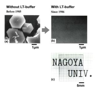
**FIGURE 8.** Scanning electron micrographs of GaN on sapphire (a) without LT-buffer layer and (b) with LT-buffer layer. (c) a photograph of specular and transparent GaN film grown on sapphire with LT-buffer layer.
