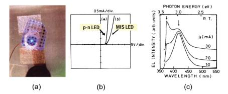
**FIGURE 14.** (a) GaN p-n junction blue/UV LEDs (black dots). An electric current is only being passed through the centered LED that is emitting blue light. (b) I-V characteristics of p-n junction LED (left) and MIS LED (right). (c) EL spectra of GaN p-n junction blue/UV LED.
