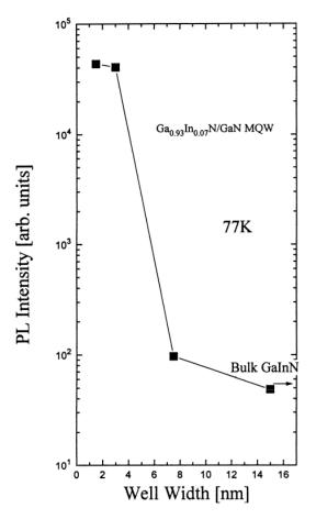
FIGURE 18. 77K PL intensities of GaInN/GaN QWs as a function of GaInN well width.
