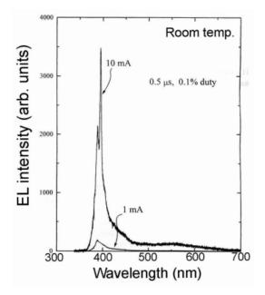
**FIGURE 19.** A stimulated emission spectrum from a GaInN/GaN QW device under pulsed current injection at room temperature.
